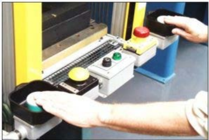
Two-hand Control on a Press
